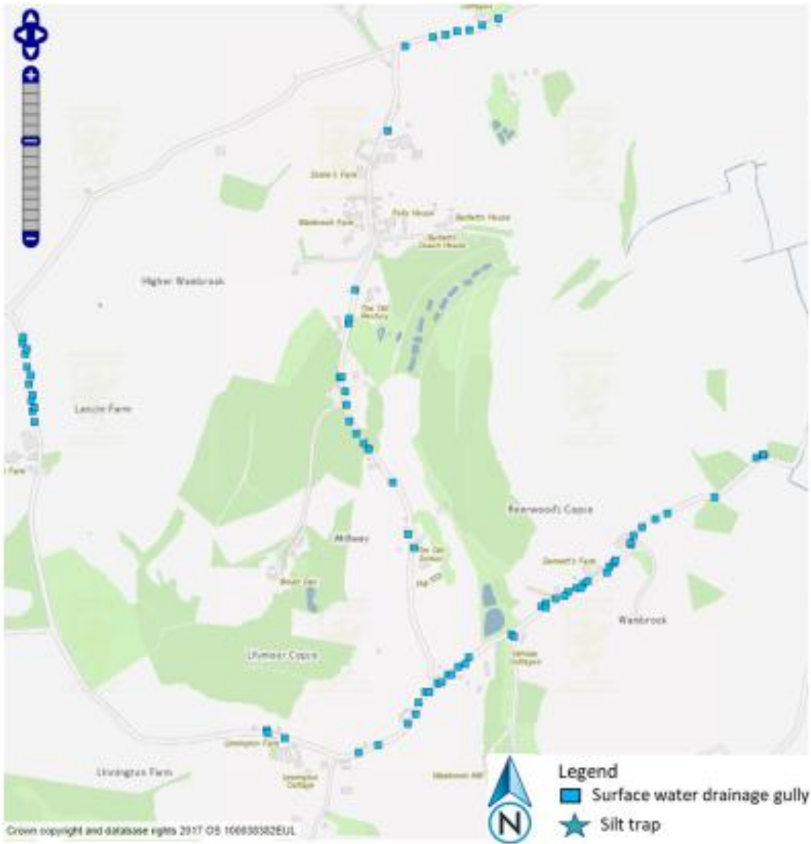
Figure 45: Highways Surface water drainage in Wambrook.
