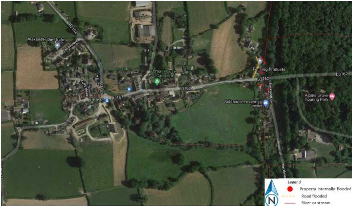
Figure 28: Flooded properties in Forton.
