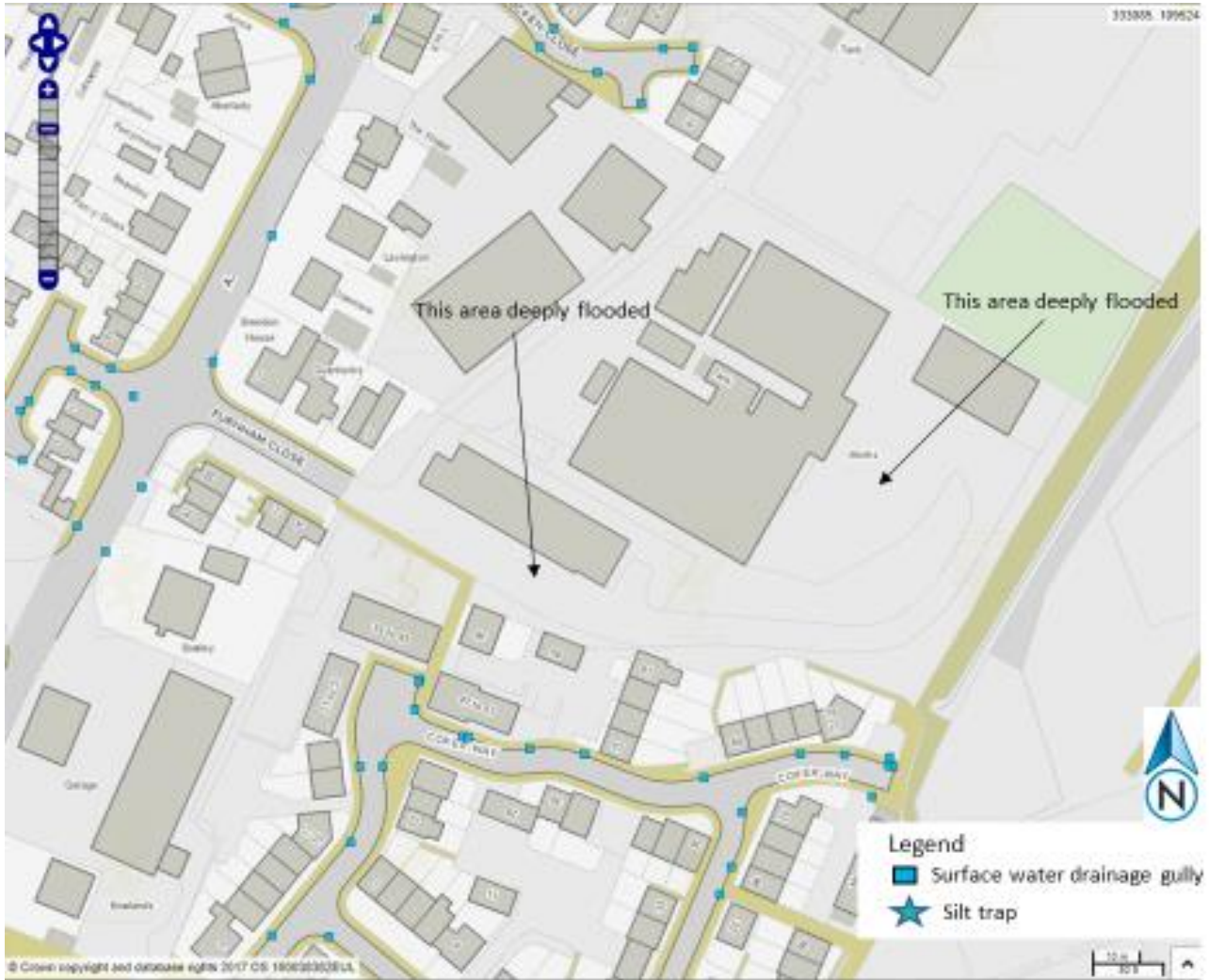
Figure 38: Highways Surface water drains in Furnham Road Industrial Estate.
